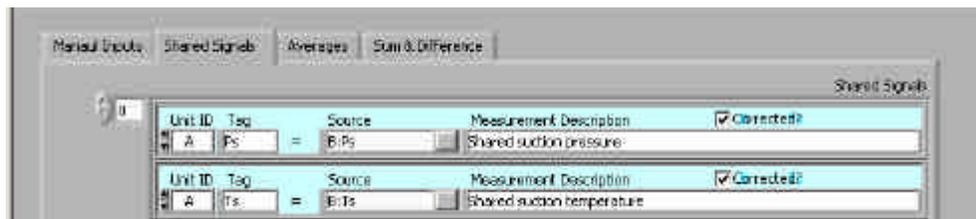
You can assign more than one tag to a signal. You can specify any PXI or manually input measurement.
