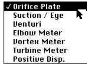
The flow measurement devices fall into two categories: those that rely on a pressure differential, and those that measure a positive displacement and generate an electrical pulse for each unit of gas which has passed through the device.
