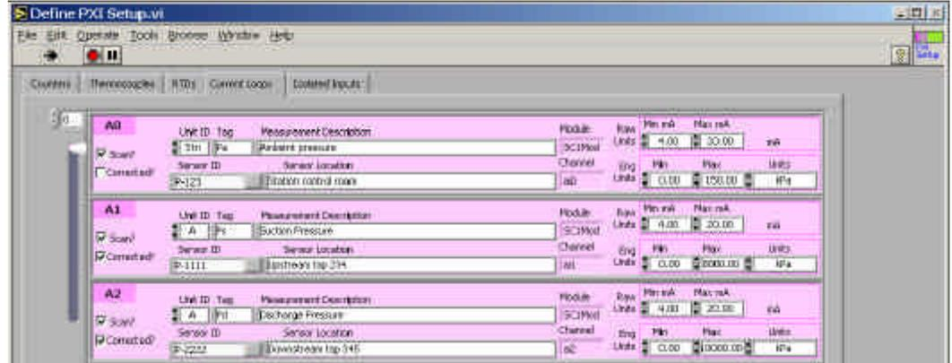
Almost anything that can be connected to a powered 4..20 mA current loop can be measured in this section (to hook up in series with an existing current loop, use the Isolated Input tab).
